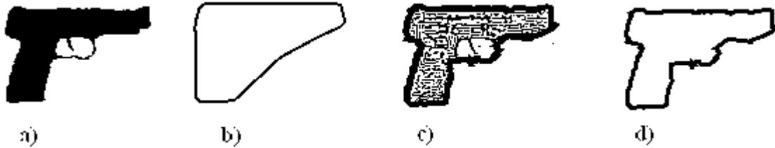
Fig. 8 a) noisy image of a pistol; b) CH; c) the image of the pistol filtered with the mask from Fig.1, and A=1 ; d) its boundary extracted with the active contour.
